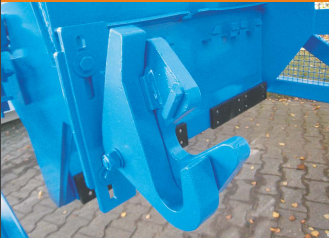
Height-adjustable and automatically locked trunnion retainer for 660-1,100 l large waste container (MGB) as per DIN EN 840
