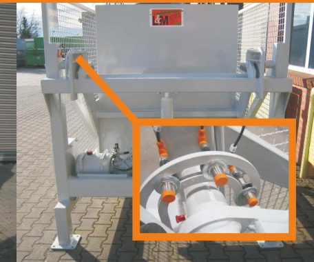
Stationary bin tipper for 660-1,100 l waste container (MGB) with protective cage and position monitoring
