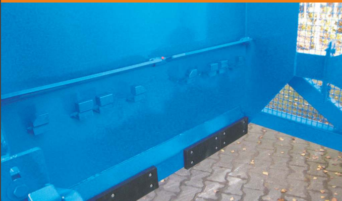
Automatically locked comb retainers for 2 x 240 l Large waste container (MGB) as per DIN EN 840
