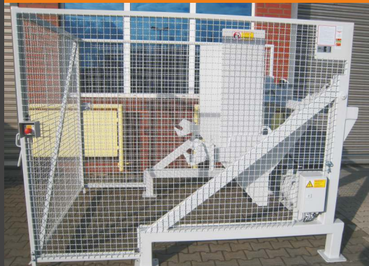
Stationary bin tipper for 660-1,100 l waste container (MGB) with protective cage and position monitoring
