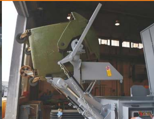
Attached bin tipper (HKV) for 2x240 l or. 1x 660-1,100 l waste containers (MGB) with automatic lid opener
