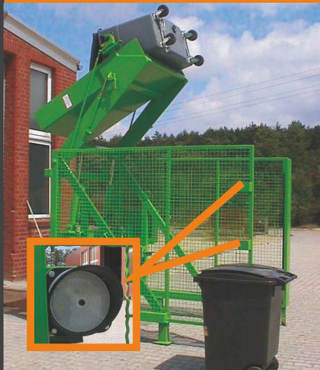
Stationary bin tipper with extended protective grid and light curtain
