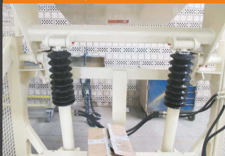
Bin tipper for the piston rods (e.g. for acidic material)
