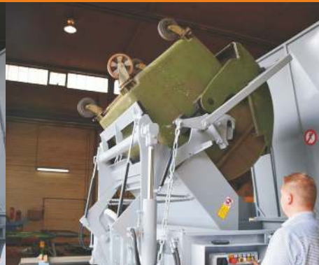
Stationary bin tipper for 660-1,100 l waste container (MGB) with protective cage and position monitoring
