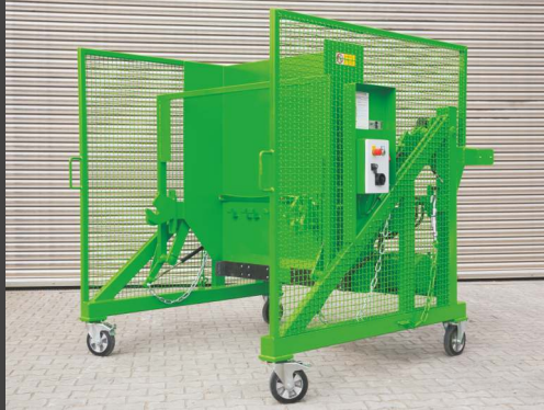
Transversally movable bin tipper for 660-1,100 l waste containers (MGB) with automatic lid opener
