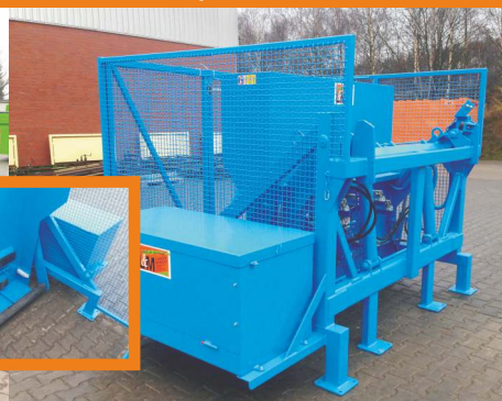
Stationary bin tipper with increased lifting force, protective cage with secured leaf door and sensor-controlled pneumatic lid opener for containers of data protection class 3
