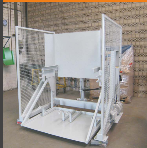
Stat. bin tipper for 2x 240 l, 1x 660-1,100 l (MGB) or several Zarges waste container
