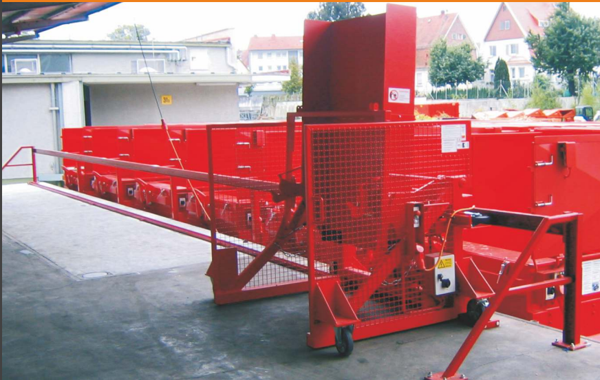
Transversally movable bin tipper for 660-1,100 l waste containers (MGB) with automatic lid opener
