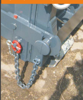
Catch rope on the discharge door to avoid accidental springing open (standard)
