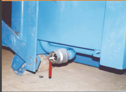
Water drain with ball valve (e.g. for liquid-tight design)
