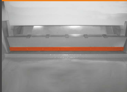
Adjustable stripper before the compaction ram (series)
