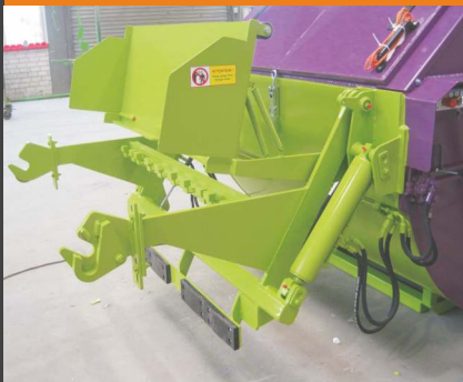
Attached bin tipper for 2x120 l or 1,100 l waste containers MGB)
