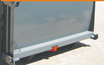
Central locking device actuated via ratchet of locking mechanism
