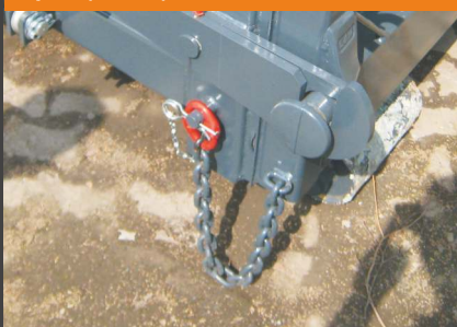
Catch chain on the discharge door prevents the door from springing open (series)
