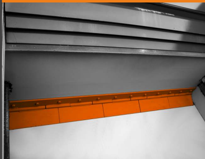
Adjustable stripper before the compaction ram (series)
