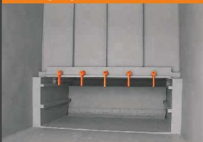
Swinging retaining teeth on the breaking edge
