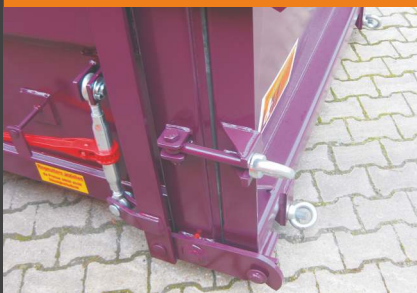
Toggle closures on the discharge opening (e.g. in case of liquid-tight design)
