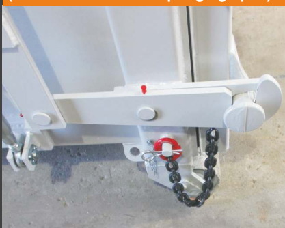
Safety chain on the discharge door (avoids uncontrolled springing open)
