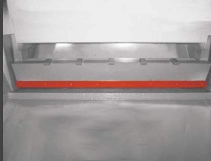
Adjustable stripper before the compaction ram
