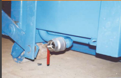
Water drain with ball valve (e.g. for liquid-tight design)
