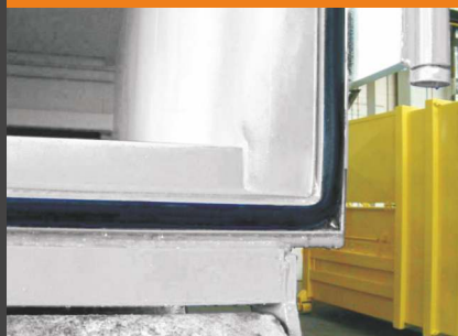
Rubber sealing on the discharge opening (e.g. in case of liquid-tight design)
