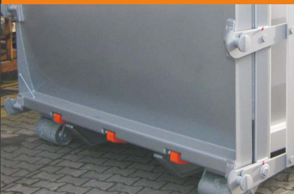
Central locking device actuated via ratchet of locking mechanism
