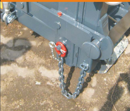
Catch chain on the discharge door prevents the door from springing open
