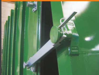
Galvanized maintenance support for pendulum flap
