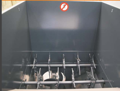
Pull-in equipment for cardboard articles above the screw conveyor
