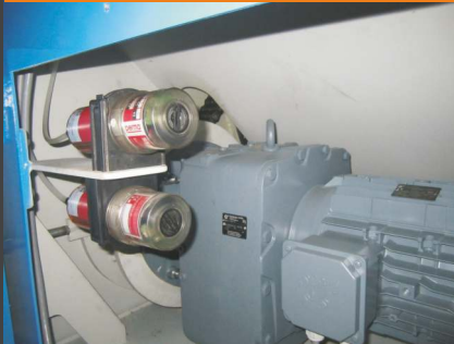
Automatic central lubrication with adjustable interval
