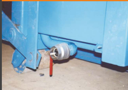
Water drain with ball valve (or screwed plug)
