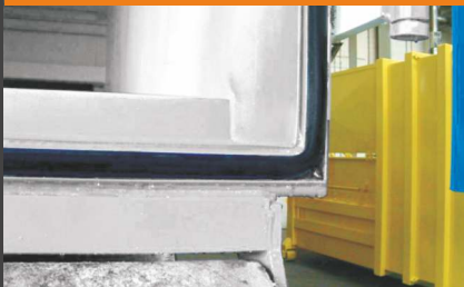
Rubber sealing on the discharge opening (e.g. in case of liquid-tight design)
