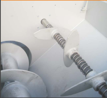
Pusher (with integrated drive) for circulation of material
