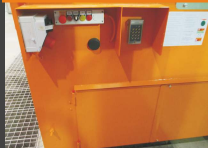
SPB LM 23 SPS with GSM warning system and PIN coded control
