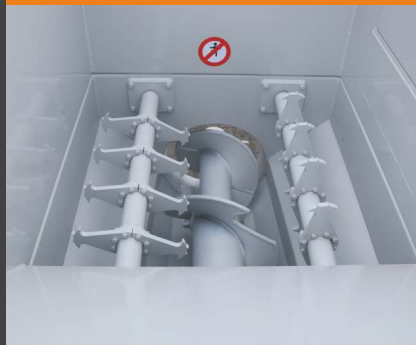
Reinforced screw conveyor and 2 x breaking shaft, design for wood crushing
