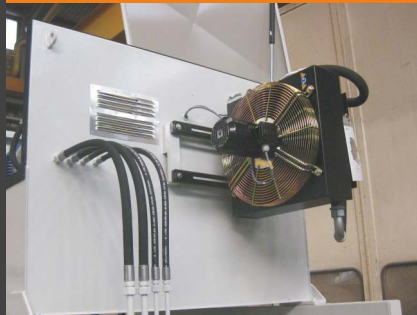
Oil cooler on external hydraulic unit
