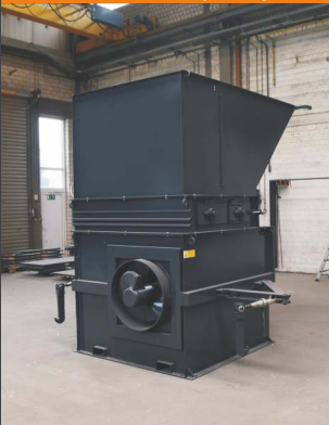
SVS 15 for PPK (with pull-in equipment for cardboard articles)
