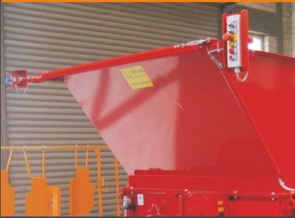
Hopper extension with emergency pull cord and remote control switch
