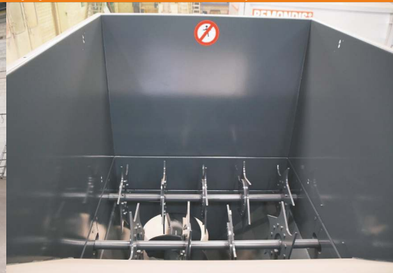
SVS 15 for PPK (with pull-in equipment for cardboard articles)
