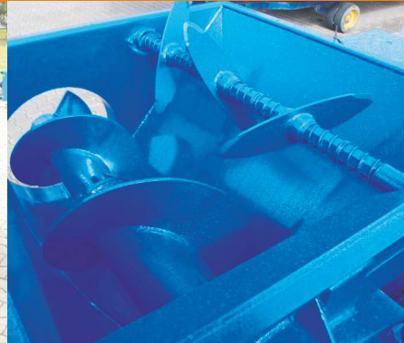
SVS 11 with pusher (for optimized drawing in of material)
