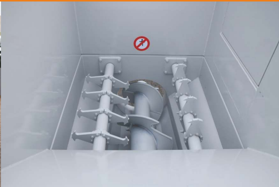
SVS 11 with pusher (for optimized drawing in of material)
