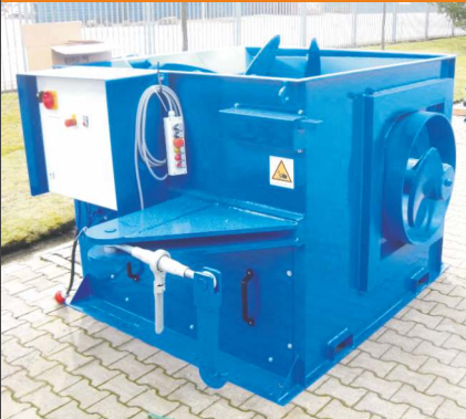
SVS 11 with pusher (for optimized drawing in of material)
