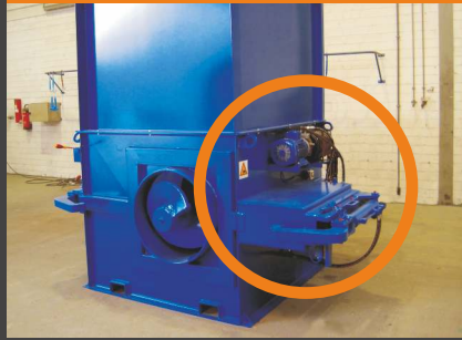
SVS 15 with hydraulic coupling (with integrated hydraulic unit)
