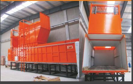
STV 10.000 with pre-chamber bulkhead and hopper design for filling from conveyor belt, designed for loading of trailers (without additional coupling)
