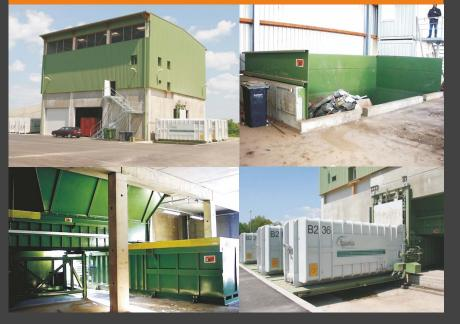
STV 10.000 with pre-chamber bulkhead and hopper design for filling from conveyor belt, designed for loading of trailers (without additional coupling)
